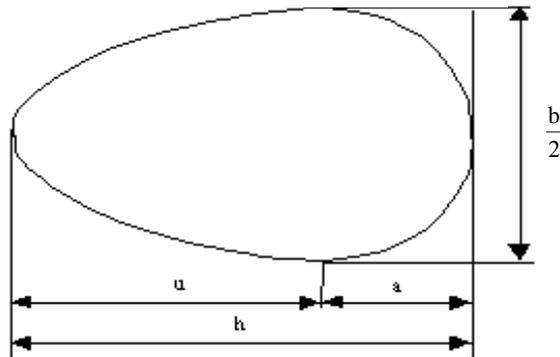
$$h := 5.8 \cdot \text{cm} \quad b := \frac{4.55}{2} \cdot \text{cm} \quad a := 2.3 \text{cm} \quad u := h - a \quad u = 3.5 \text{cm}$$
