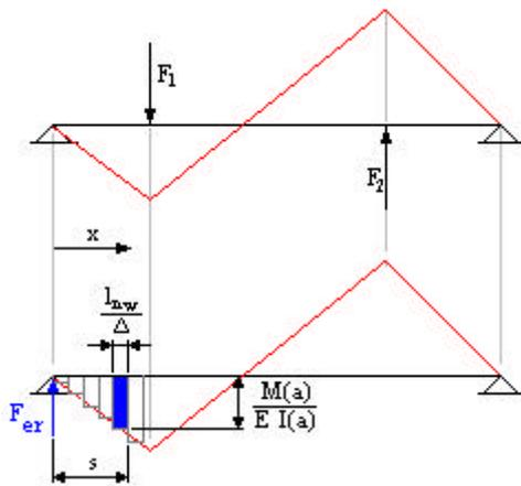
$$F_{er} := \frac{\sum_{x=0}^{\Delta} \frac{M \left( x \cdot \frac{\text{liter}_{n_w}}{\Delta} \right) \cdot \frac{\text{liter}_{n_w}}{\Delta} \cdot \left( \text{liter}_{n_w} - x \cdot \frac{\text{liter}_{n_w}}{\Delta} \right)}{E \cdot I \left( x \cdot \frac{\text{liter}_{n_w}}{\Delta} \right)}}{\text{liter}_{n_w}}$$
